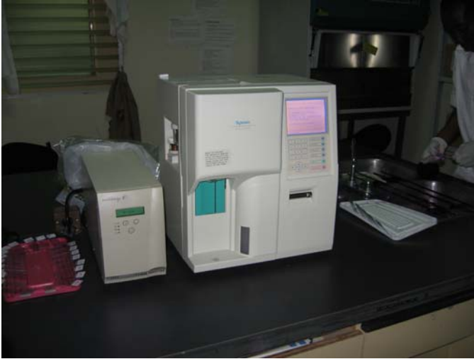
Point-of-use UPS systems are recommended for all sensitive equipment
